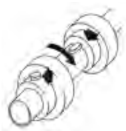
Illustration 10 - protrusions can cause injury from entanglement
