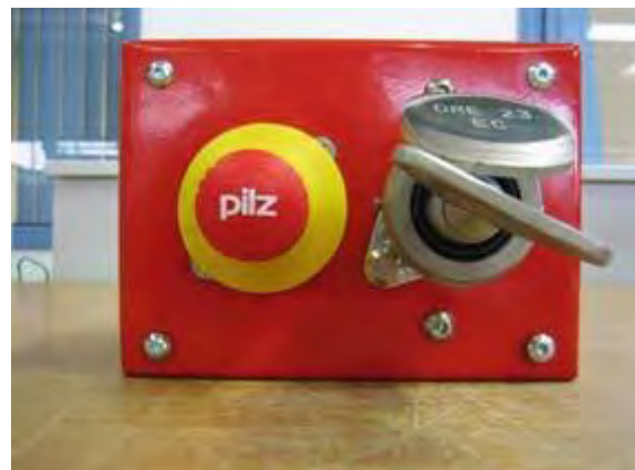
Captive key systems: The key cannot be removed unless it is in the off position. The same key is used to unlock the access gate. Only one key per system is retained by the locking mechanism.
