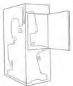
Illustration 12 - An example of a hinge door guard (interlocking movable guard)
