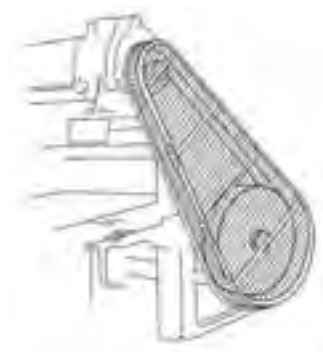
Illustration 18 - Fixed guard for a pulley and drive constructed of wire mesh and angle section preventing access to transmission machinery
