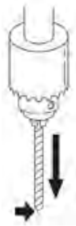
Illustration 7 - stabbing points caused by moving parts of machinery or material
