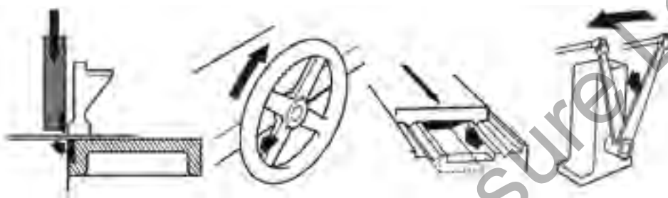
Illustration 3 – shear points between a machinery part and a work piece
